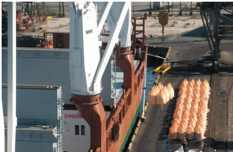
**Figure 2:** Loading of the raw material in the big-bags onto the bulk carrier.
