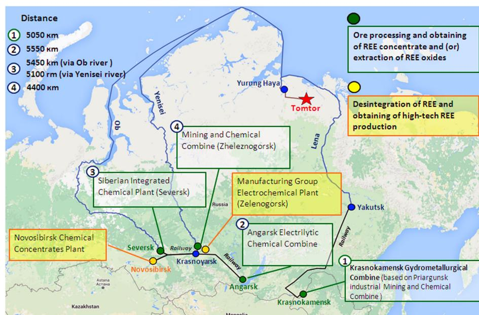
**Figure 1:** Options for the transportation of the ore and collective carbonates to the processing and enrichment enterprises.
